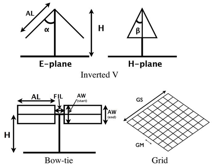
Fig. 1. Geometric parameters considered in the EM simulation with NEC: arm length (AL), arm width (AW), height (H), droop angle  $\alpha$ , apex angle  $\beta$ , grid size (GS), grid meshing (GM). Electrical parameters: conductivity  $\sigma$ , dielectric constant  $\epsilon$  for various types of ground.
