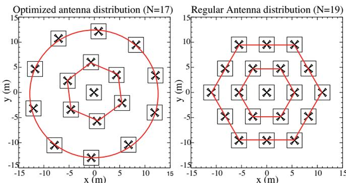
Fig. 2. Minimal distance between antennas is  $d=5.5m$ . (Left) Cluster of  $N = 17$  optimized for low SLL with simulated annealing method. It is composed of a central 6-antenna hexagon and a 10-antenna ring. (Right) Regular array of  $N = 19$  antennas composed of two concentric hexagons.
