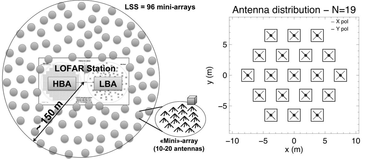
Figure 1: Left: The LOFAR Super Station is a set of 96 mini-arrays (or tiles) of 10-20 antennas analog-phased, spread around the Nançay international LOFAR Station within a range of  $\sim 150$  m. Right: Possible antennas distribution within a mini-array, here with  $N = 19$  elements arranged on an hexagonal grid. This distribution is a good compromise between an axisymmetric distributions (ensuring a low sidelobe level) and a regular array (providing easy analog phasing) (see 3.2).
