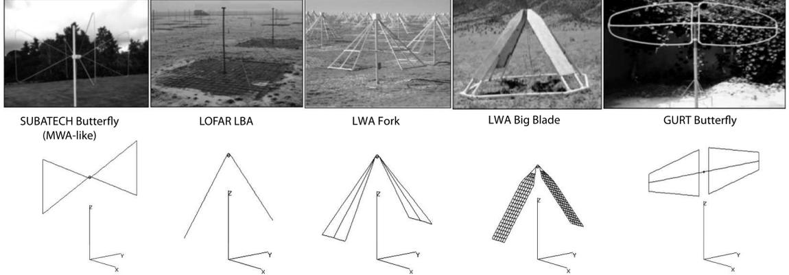
Figure 2: The top panel displays the linearly polarized dipoles that have been studied in Nançay. The bottom panel displays their numerical wire model as used in input of electromagnetic simulations with NEC – see text.
