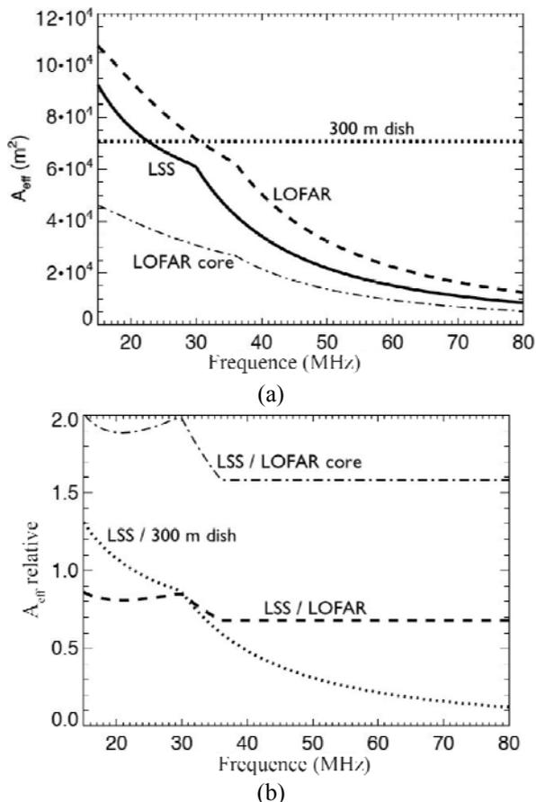
**Fig. 4.** Theoretical absolute (a) and relative (b) effective collecting areas of NenuFAR between 15 and 80 MHz for NenuFAR (NenuFAR), the full LOFAR-LBA, the LOFAR core only and a typical 300m-diameter dish radio telescope (Arecibo).
